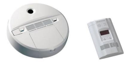
CO alarms come in a variety of types. There are wall and ceiling mounted units that look similar to a smoke alarm. These units can be battery powered or hardwired electric with a battery backup There is also an electric type, some with a battery backup, that plug directly into an electrical outlet, The only requirement of the code is that the CO alarm comply with UL 2034. Look for the UL listed label on the alarm to verify its compliance with the UL 2034 standard.
